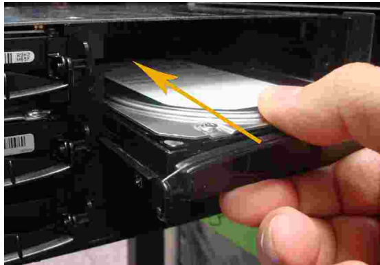
Figure 3-14: Loading a disk drive (Nexsan E18X top; Nexsan E32X bottom)
