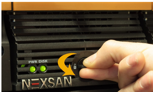
Figure 3-5: Unlocking the drive drawer
