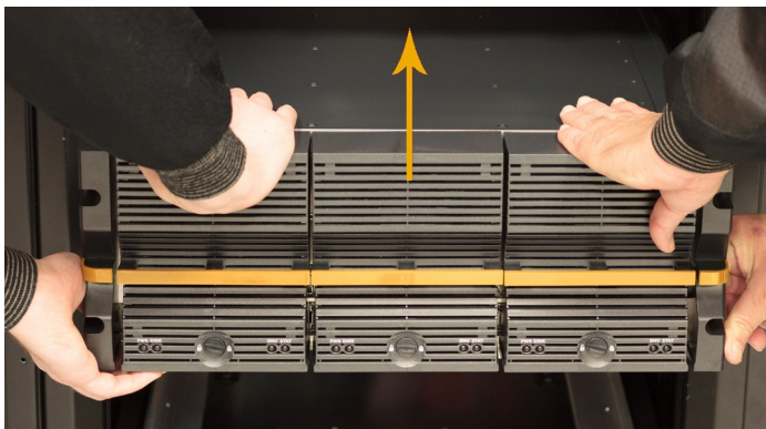
Figure 3-1: Sliding the Nexsan E60X/Nexsan E48X onto the mounting rails
