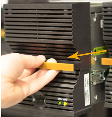
Figure 3-6: Sliding the drive drawer out
