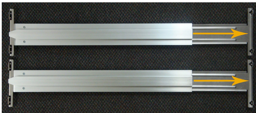
Figure 2-10: Extending the rack-mount rails
