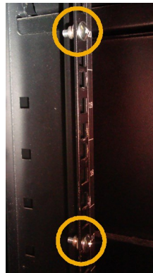
Figure 2-12: Attaching the rear rack nuts
